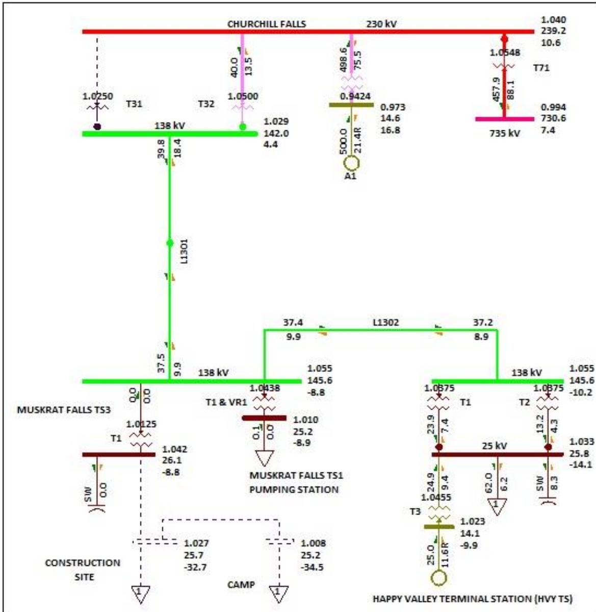
Figure 6 62 MW Transfer with Churchill Falls T31 Out of Service
