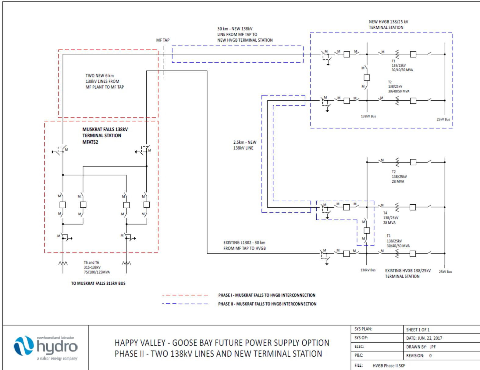
Figure 15 Phase II – Double 138kV Transmission Interconnection to Happy Valley-Goose Bay
