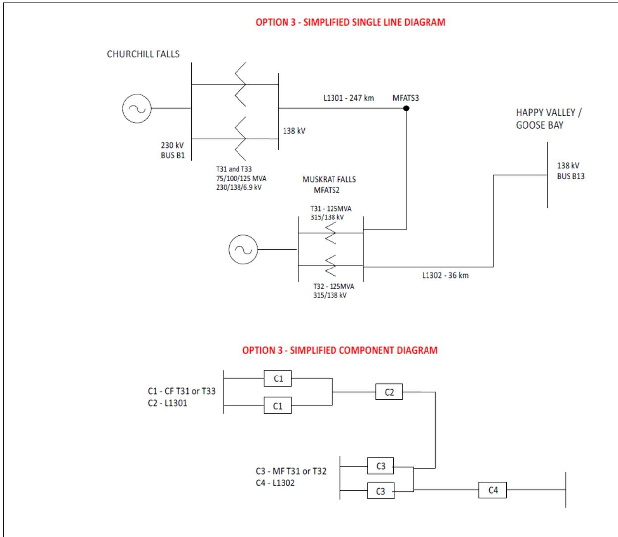
Figure K.3 Option 3 Simplified Single Line/Component Diagram
