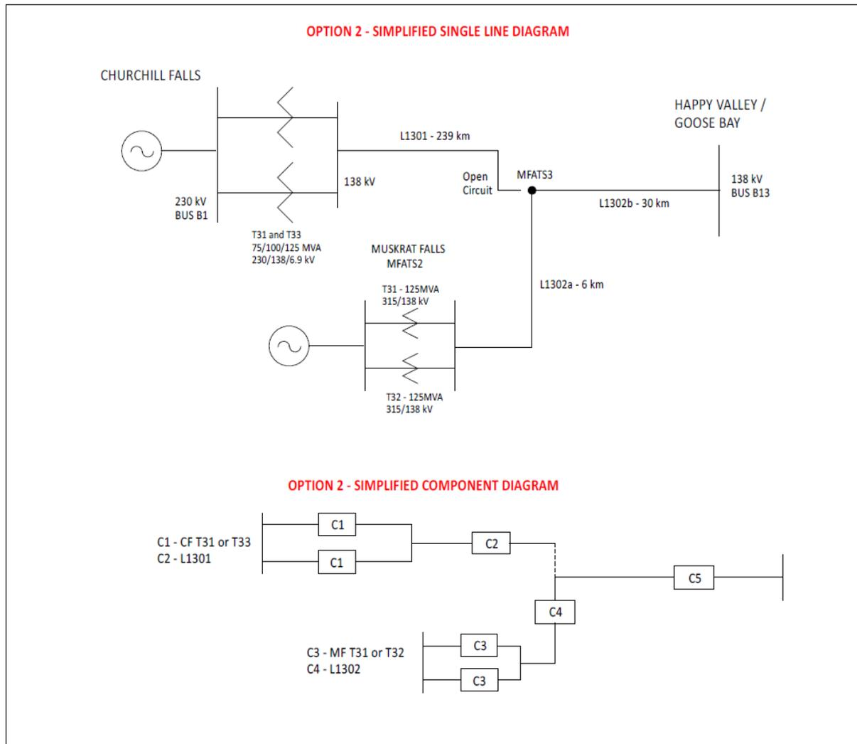
Figure K.2 Option 2 Simplified Single Line/Component Diagram
