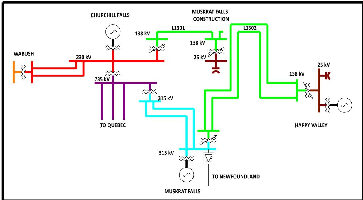
**Figure 12 Option 4 Transmission Configuration**
