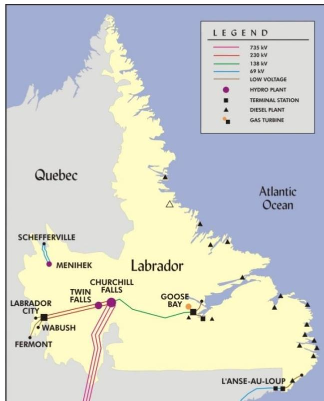
Figure 1 Labrador Interconnected System
