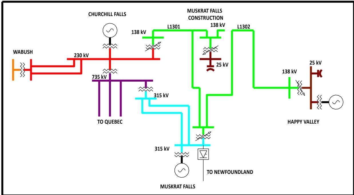
**Figure 11 Option 3 Transmission Configuration**
