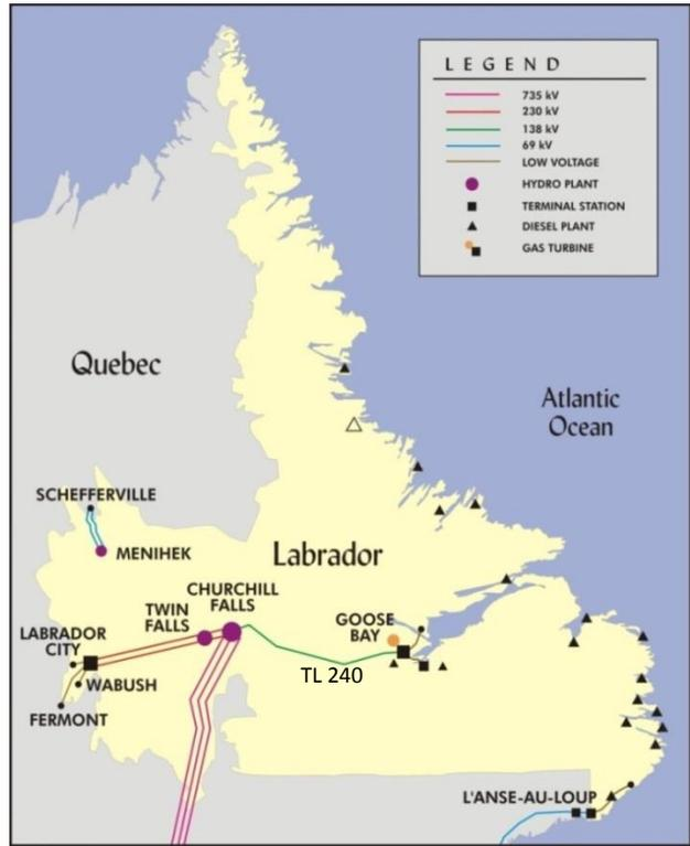
Figure 4 Labrador Interconnected System
