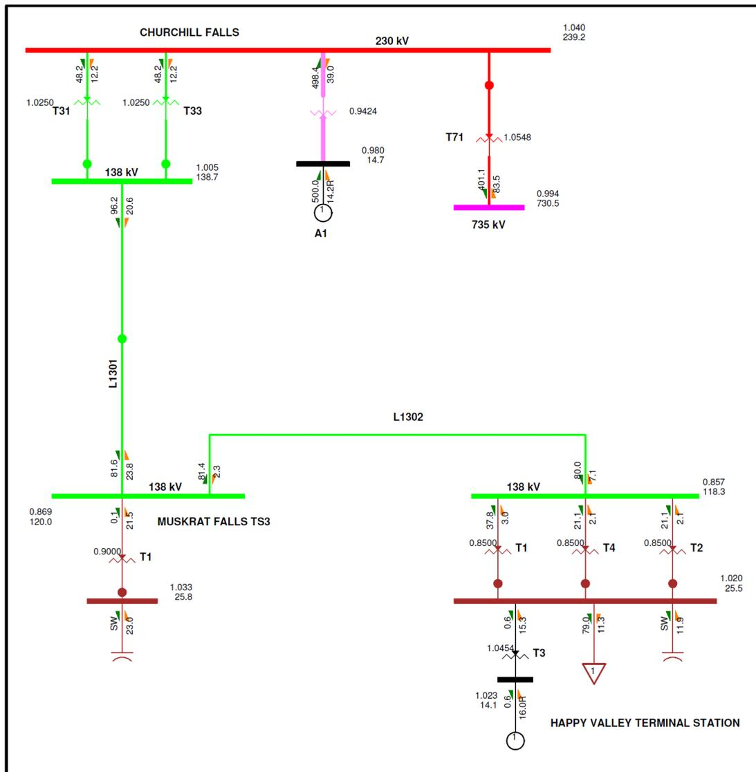
Figure 7 79 MW Transfer with Additional Churchill Falls 125 MVA Transformer
