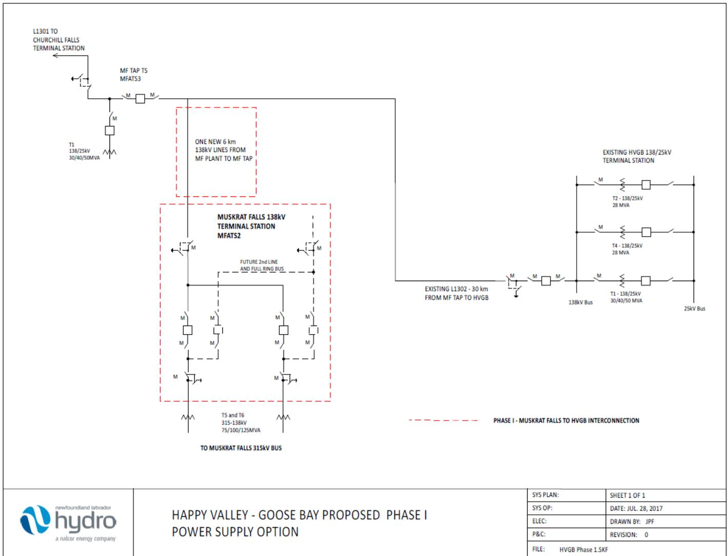
Figure 2 Electrical System for Upper Lake Melville Area – Phase I
