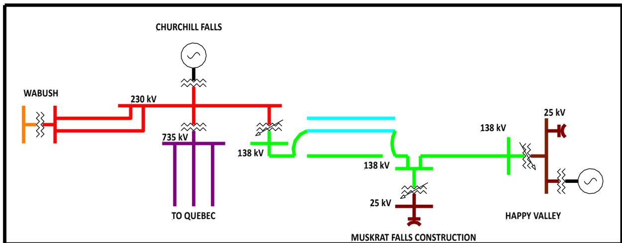
**Figure 4 Labrador Interconnected System 2017-18 Peak<sup>4</sup>**
