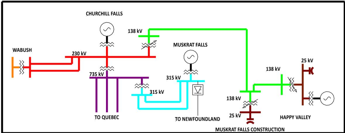
Figure 1 Labrador Interconnected System with Muskrat Falls Complete
