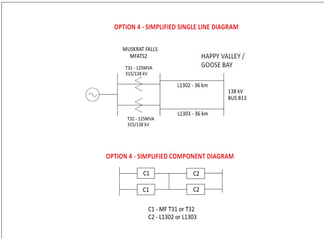
**Figure K.4 Option 4 Simplified Single Line/Component Diagram**
