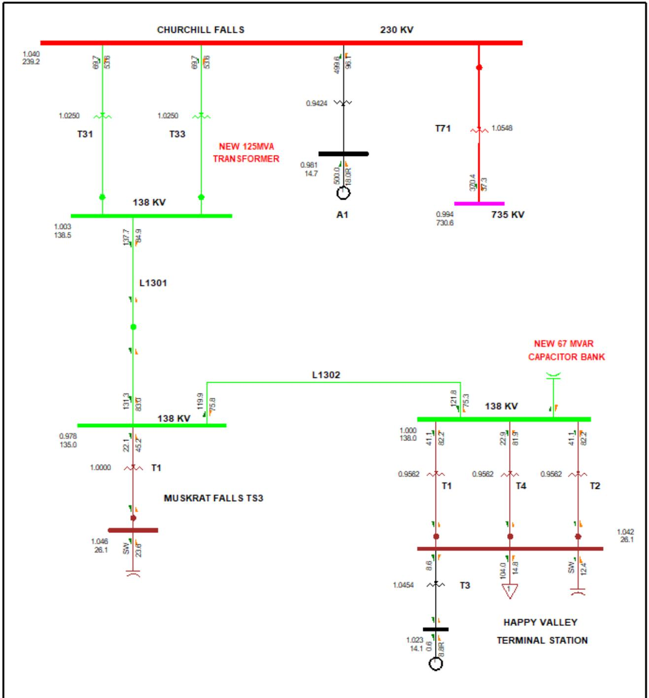
**Figure 8 104MW Transfer with Additional 67 MVAR Capacitor Banks at Happy Valley with one 138/25 kV, 30/40/50 MVA Transformer Out of Service**
