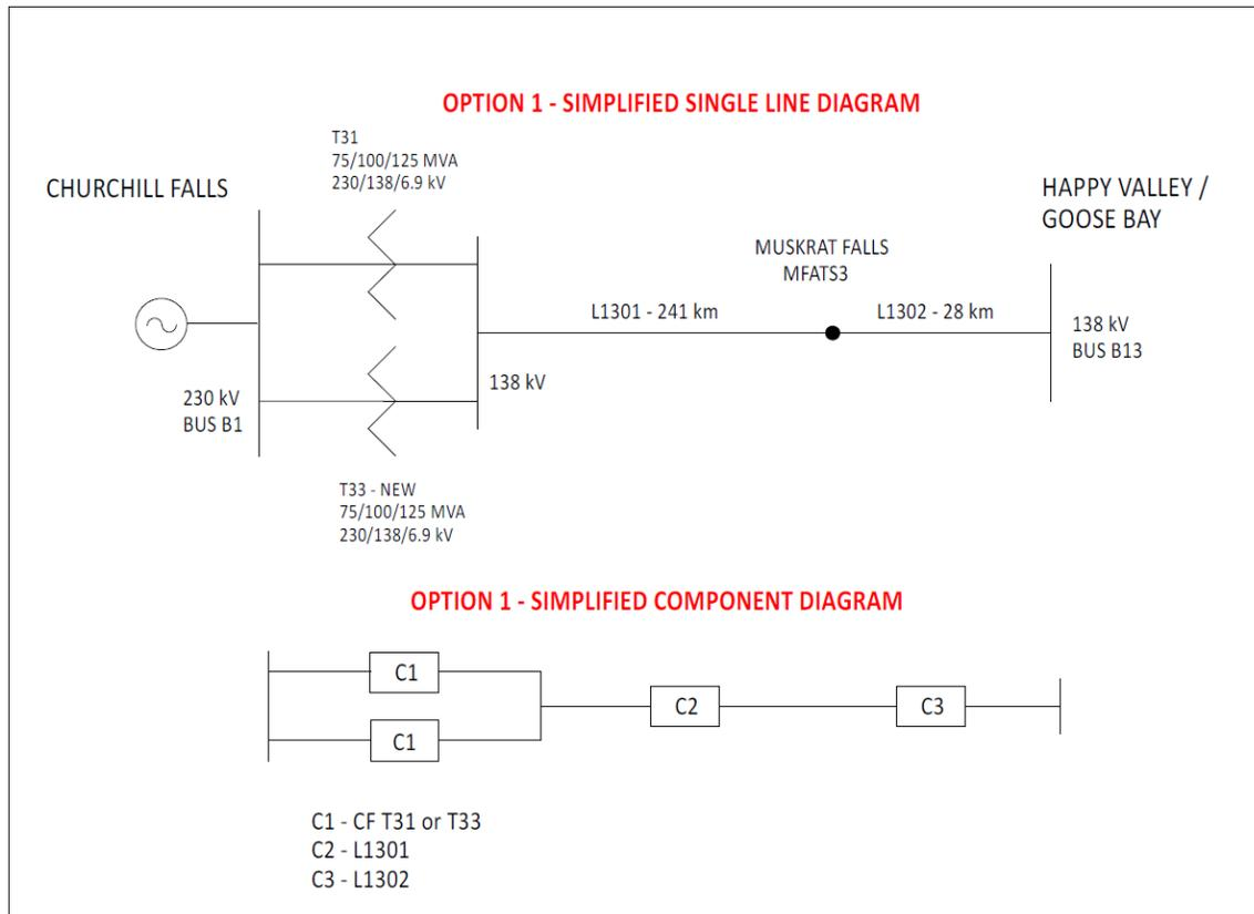
Figure K.1 Option 1 Simplified Single Line/Component Diagram
