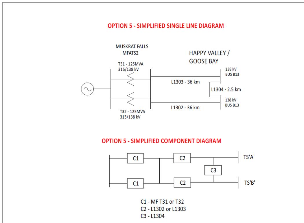
**Figure K.5 Option 5 Simplified Single Line/Component Diagram**
